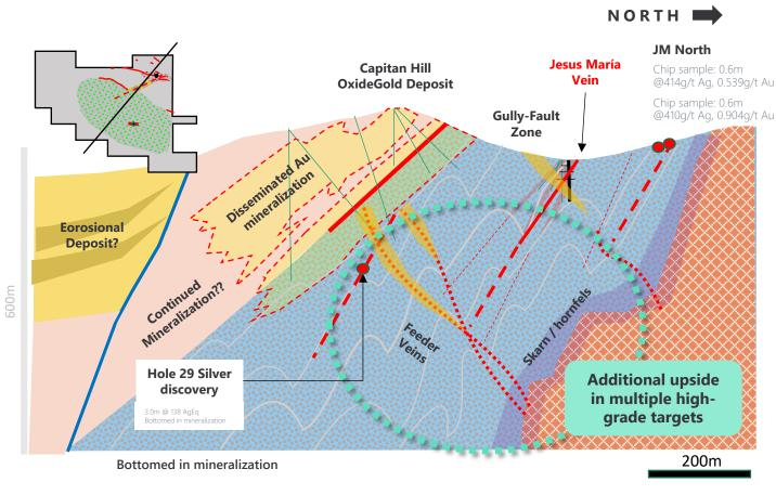
Schematic illustration of Cruz de Plata mineral system showing different styles of mineralization identified.
